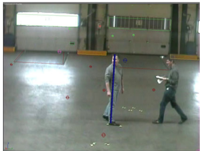
FIG. 5—Example of the 3D model projected onto an image. A cylinder is used to measure the height of the person.
